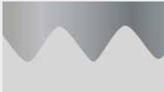
Pre-drilling Ø 17.1 mm
