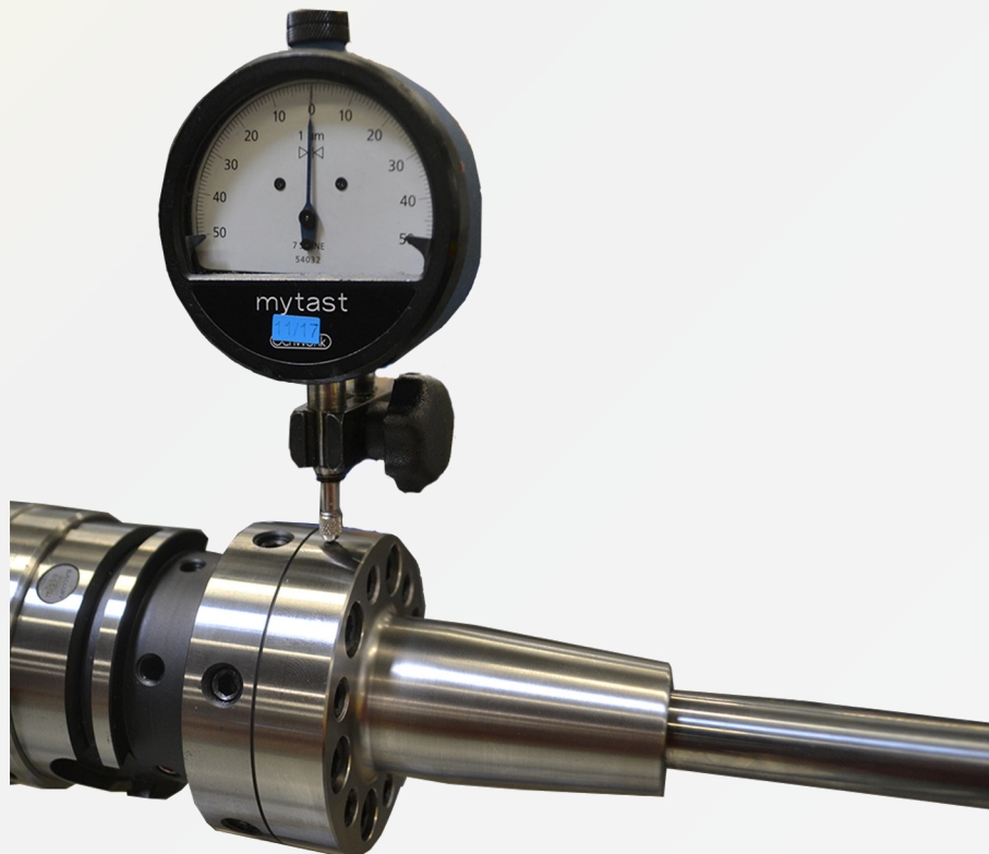
Fig. 8: Positioning the dial indicator at the concentricity checkpoint
