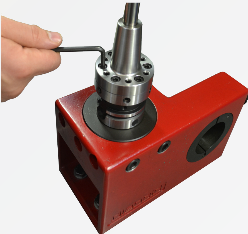
Fig. 6: Slightly tighten the fastening screws
