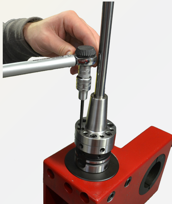
Fig. 7: Tightening the fastening screws with torque
