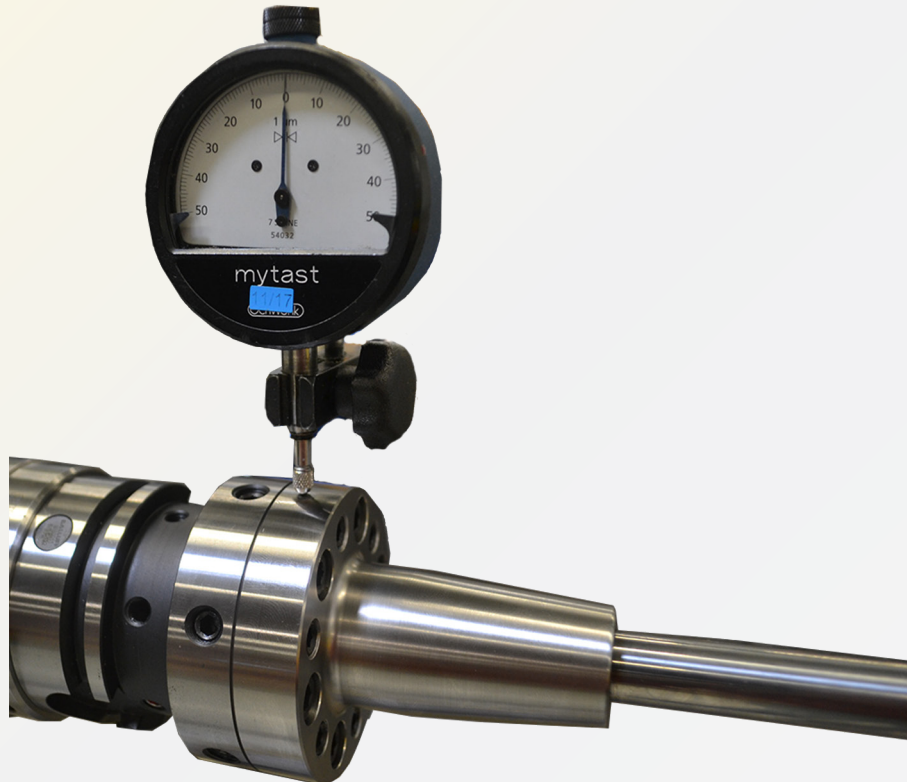
Fig. 18: Checking the radial alignment of the module flange
