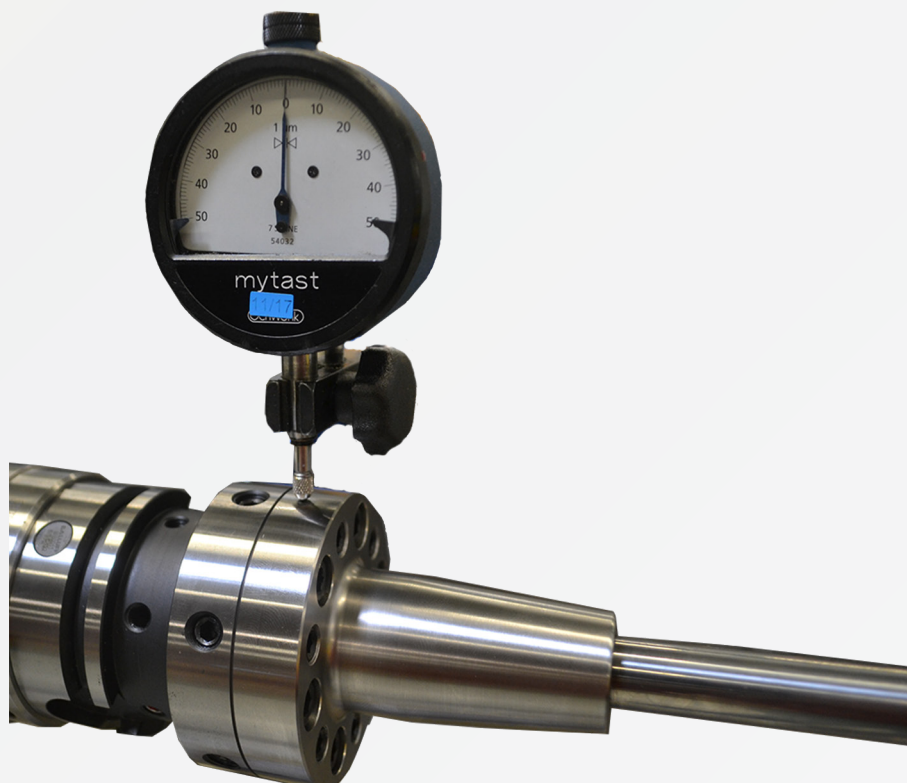
Fig. 10: Setting the dial indicator to zero
