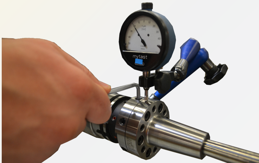
Fig. 11: Adjusting the concentricity error
