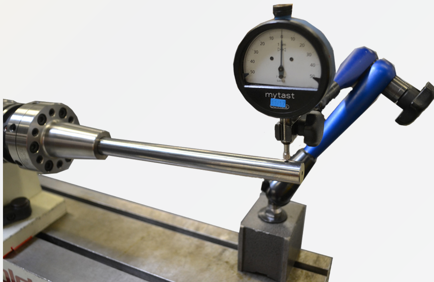
Fig. 14: Position the dial gauge at the front concentricity checkpoint
