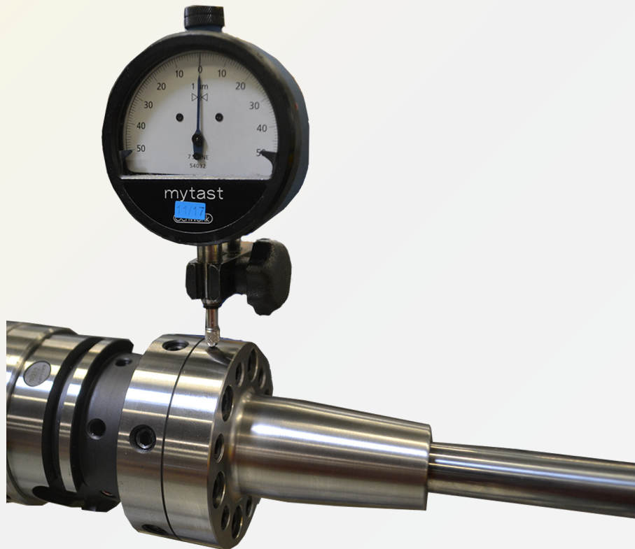
Fig. 13: Checking the concentricity error
