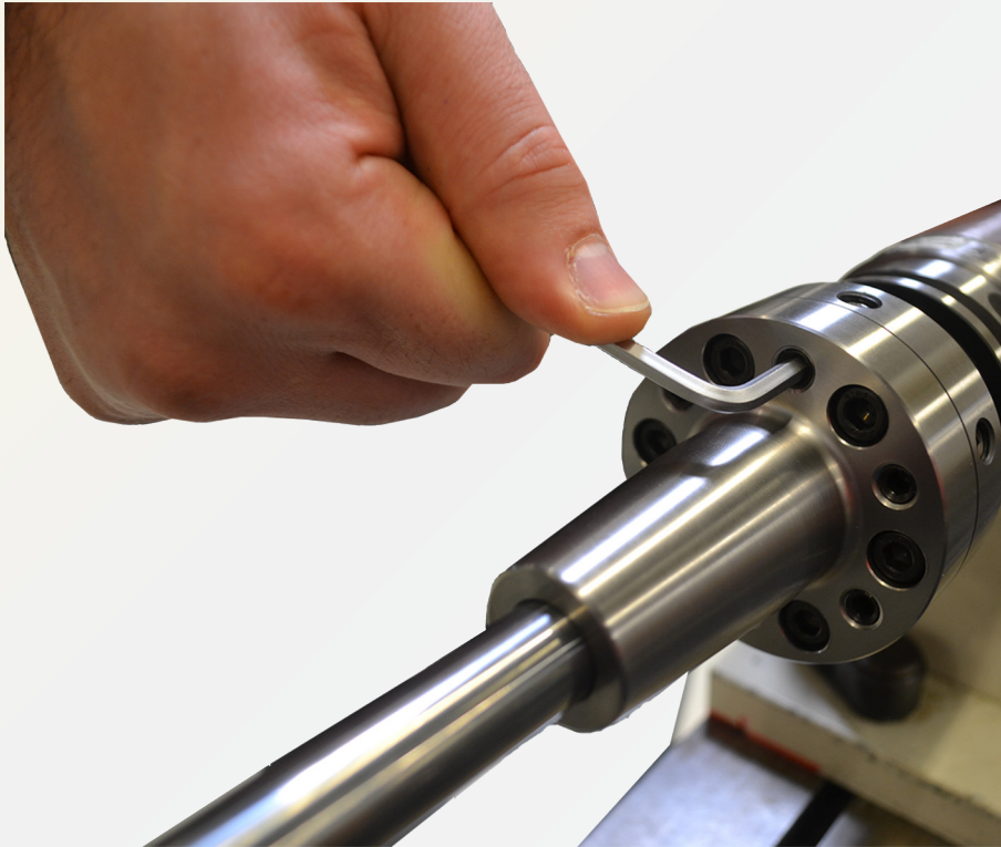
Fig. 17: Aligning the angle with the angle adjustment screws
