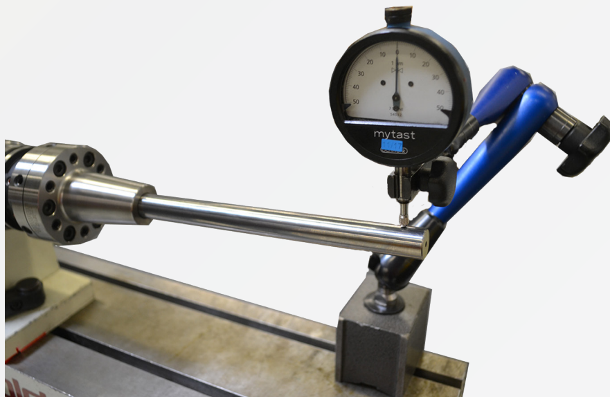
Fig. 16: Setting the dial indicator to zero
